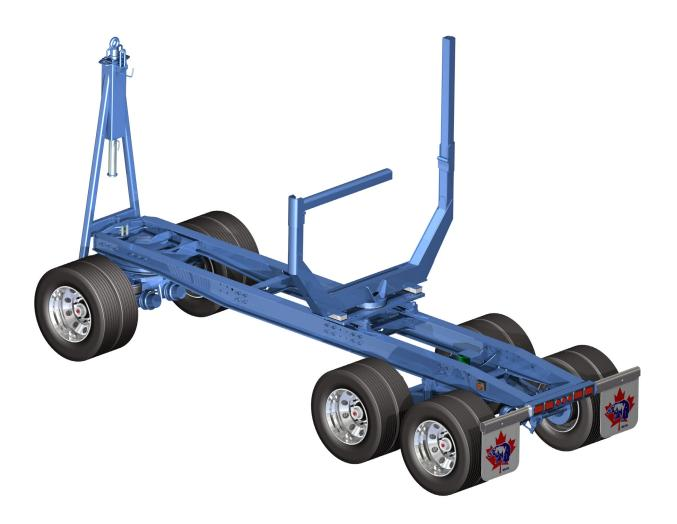
Chassis: Heavy Duty QT-100 frame, QT-100 cross members. "Huck" bolt fasteners for cross-member locations.
