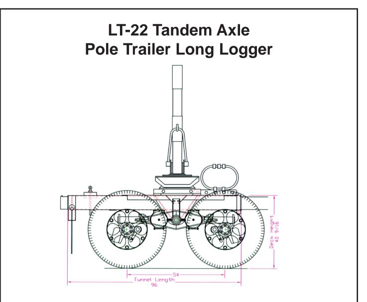
Features: One Piece Top Deck. Intergal Out-Board Legs. Heavy Duty Hi-Tensile Trunnion Shaft. Urethane Bushing in All Suspension Locations. 2 Piece Walking Beam End Caps. Sintered Bronze Filters on Service and Emergency Air Lines. Low temperature "Arctic Grade" reach air lines. One Piece Sealed Electrical Light Cord. Various Bunk, Bolster, Scale, Hub/Drum, Tire and Rims Options.
