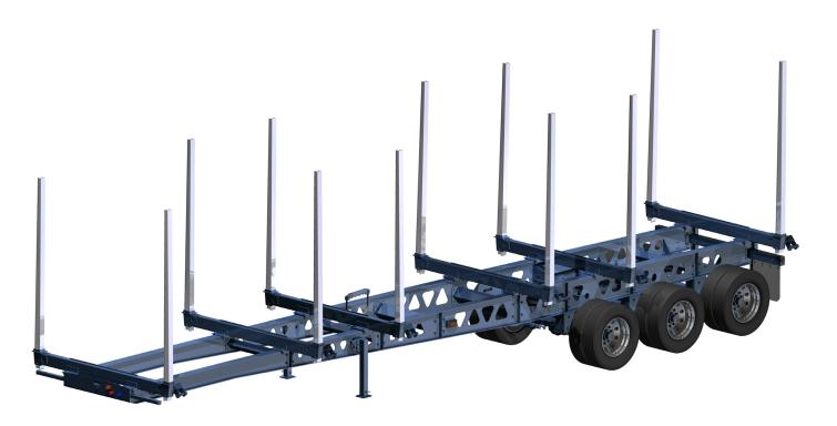
Chassis: Heavy Duty Long NeckQT-100 frame, HD Angled cross members. Swing-Up Pin-Type landing gear.
