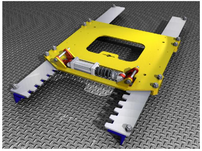
3" Travel Increments, From 24" to 144". Tapered Notches Eliminates Play. Air to Unlock Spring to Lock. Can be Configured with Air to Lock. Open Rail Design Allows Easy Service. Vertical Jaw Contact and Hinged Surfaces Eliminates Material Build-Up Allowing Movement in Adverse Conditions. UHMW Slide Plates for Easy Slide Under Load. Accepts Holland XA7800 series Pedestal, Vulcan L04,L11 and L27 Load Cells, S.I. Titan and Titan II Load Cells. (AML2420) shown
